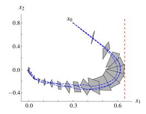
Fig. 1. The dark shaded regions show selected cross-sections of an optimized polytopic tube and the red dashed line shows the state constraint  $\mathbb{X} = \{y \mid y_1 \leq 0.65\}$ . Left: The black dashed line depicts the disturbed closed-loop trajectory for a traditional MPC controller, which violates the state constraint. Right: The blue dashed lines show closed-loop trajectories for three selected uncertainty realizations.
